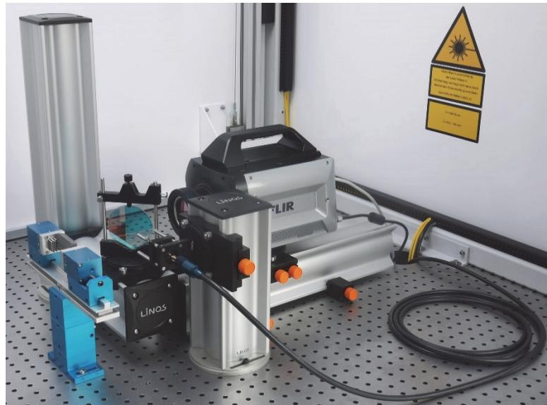
**Fig. 2:** Lab setup of Forakam: FLIR X6901sc, LTvis 250 NT diode laser fibre, dicroitic mirror and sample in clamping system.
