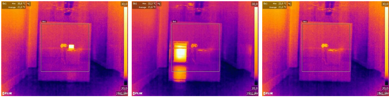
Fig. 4. IR pictures of second session of glass object at 2,5m distance with (left) concrete block hot spot; (middle) heating plate hot spot; and (right) without hot spot
