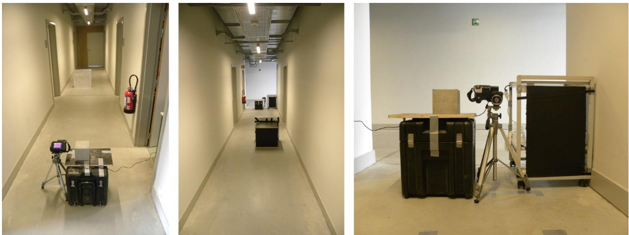
Fig. 3. Measurement set-up in corridor: (left) view from IR camera to object; (middle) view from object to IR camera; (right) positioning of concrete block and heating plate next to IR camera
