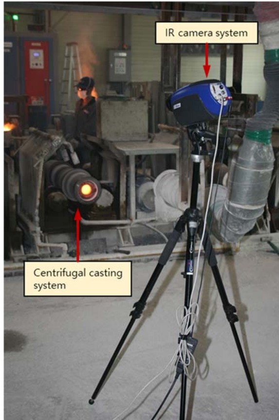
Fig. 3. Experimental setup for monitoring temperature variation
