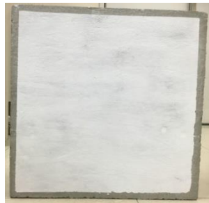
Fig. 6 Specimen with simulated discoloration, prepared by applying Ca(OH) 2 solution to concrete surface (shown in Fig. 2).
