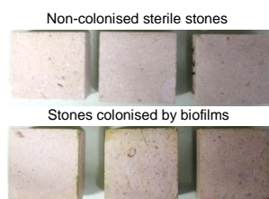
Fig. 8. Samples testing in pulsed IRT. The upper samples are controls without biological colonisation, the lower ones are colonised at 6 months of exposure. Photo in natural light.
