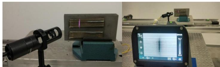
**Fig. 2:** Experimental set up showing the laser line and the test sample.
