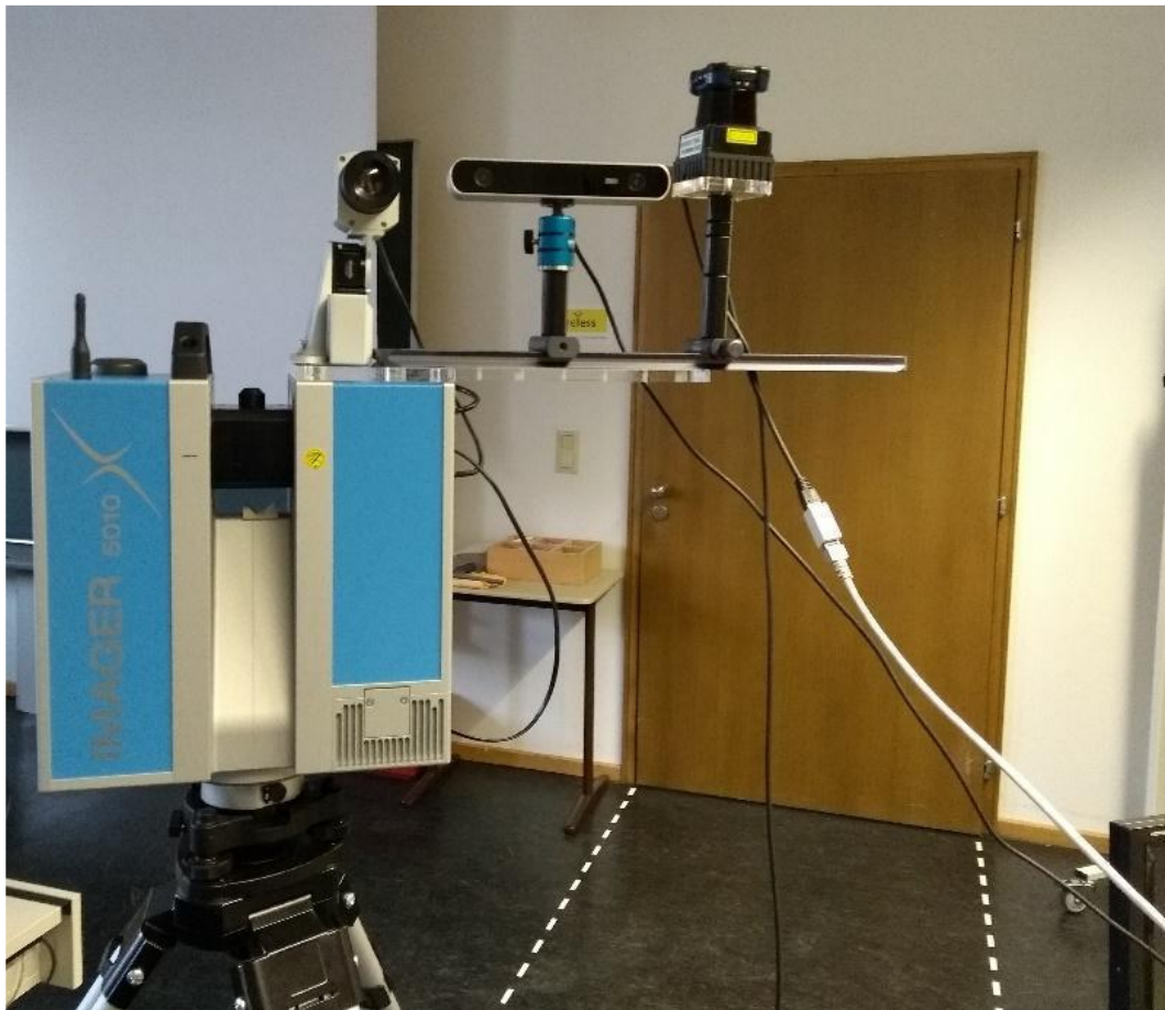
Fig. 4: Sensor rig with all sensors. Relative orientation of the TIR and RGB camera and the laser range scanner with the Z+F laserscanner as origin of the coordinate system
