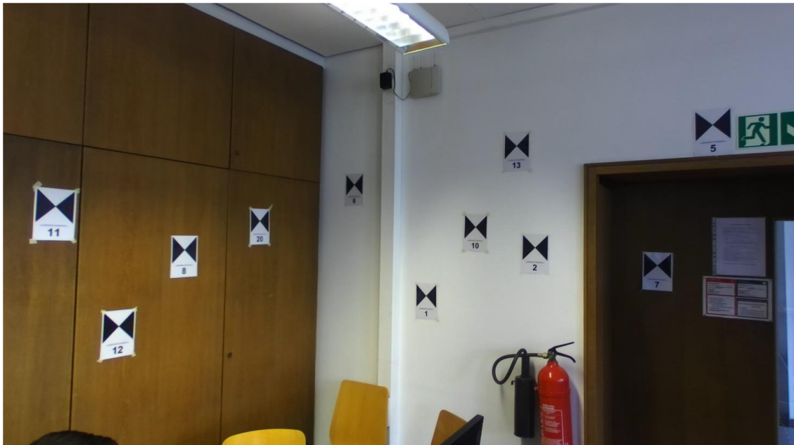
Fig. 1: Targets used for sensor registration.
