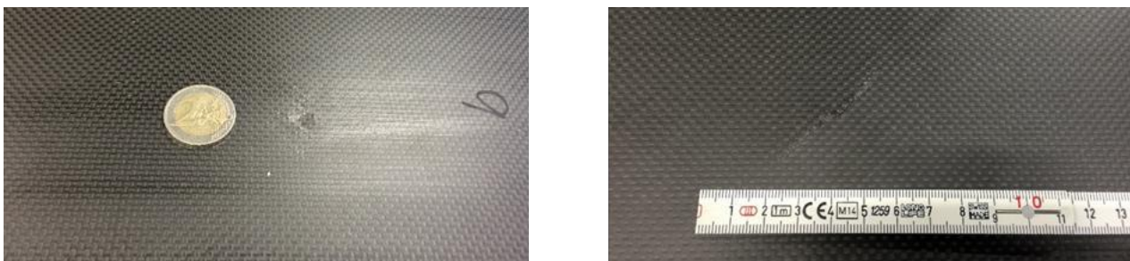
Fig. 3. Impact damage in CFRP: Front surface damage on the left, rear surface on the right.
