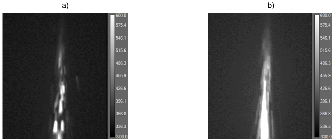
Fig. 12. Comparison of images obtained with SWIR camera for ET – 0.2 ms and f/1.4: (a) with shielding gas, (b) without shielding gas
