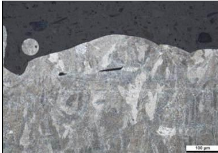
Fig. 6: Metallography of a lack of fusion defect
