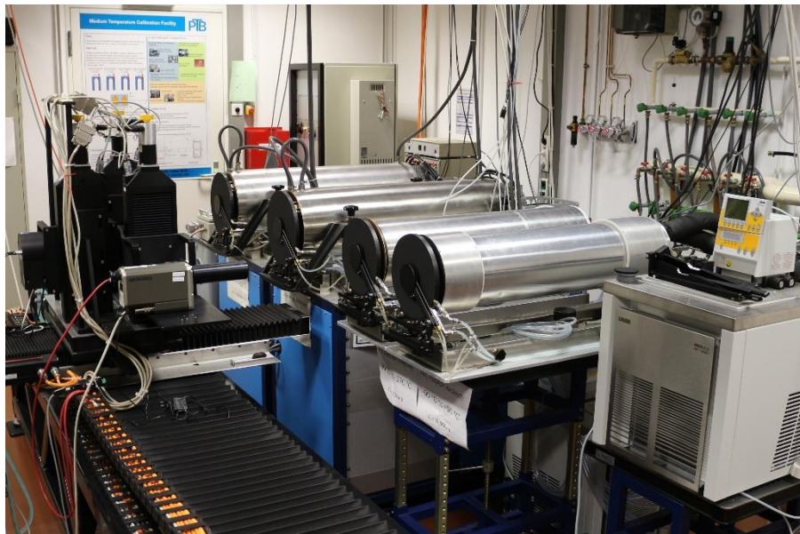
Figure 1 Germany's national standards for radiation temperatures from -60 °C to 962 °C.
