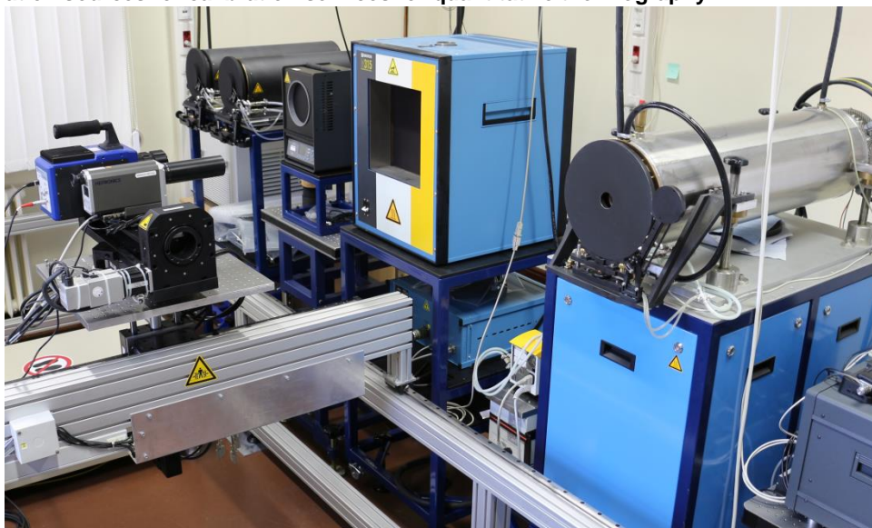
Figure 2 The calibration facility for thermal imagers.
