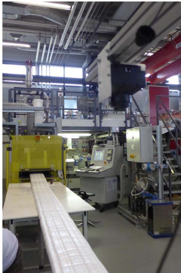
Fig. 2: Passive thermography at the pilot extruder of Fraunhofer ICT
