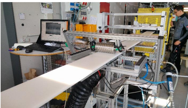
Fig. 13: Machine for an automated and reproducible application of the cooling fingers
