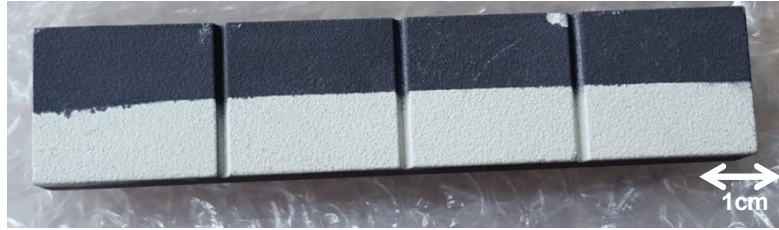
Fig. 1. Photo of zirconia coated IN 738 sample. Dimensions: 89 mm x 19 mm x 9 mm. Upper half is additionally sprayed with graphite.
