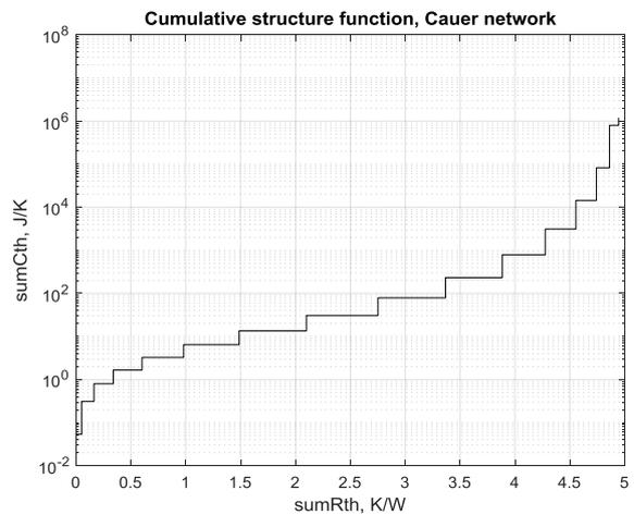
Fig. 6. Cumulative structure function for the thermal impedance (15)
