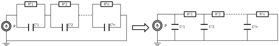
Fig. 2. Foster and Cauer thermal networks
